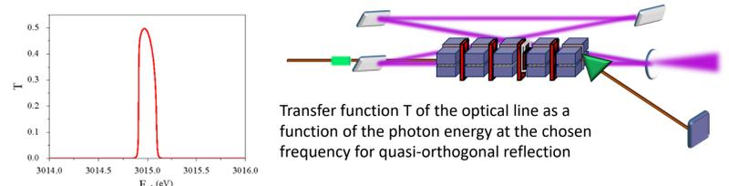
The cavity contains three diamond mirrors and one beam splitter, operating at 4.17 Å.
