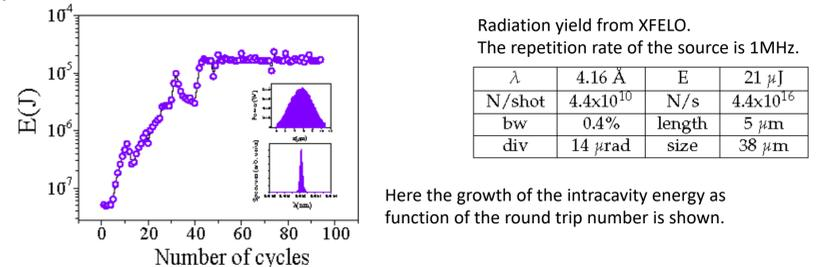
Radiation yield from XFEL. The repetition rate of the source is 1MHz.
