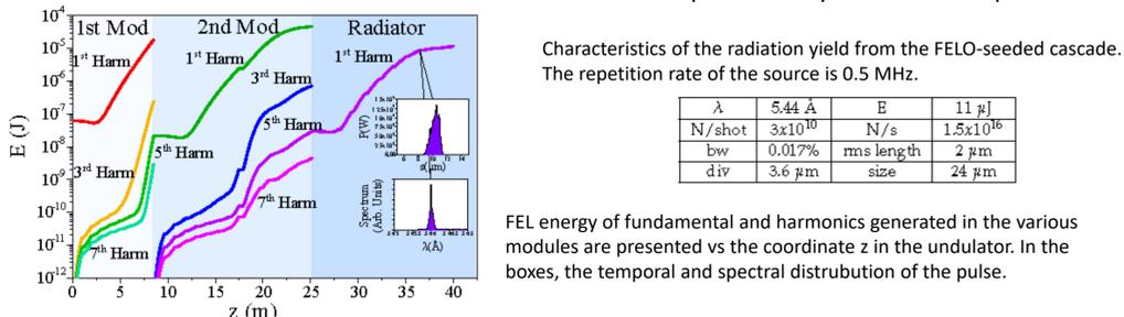
Characteristics of the radiation yield from the FELO-seeded cascade. The repetition rate of the source is 0.5 MHz.
