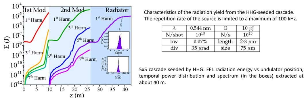
Characteristics of the radiation yield from the HHG-seeded cascade. The repetition rate of the source is limited to a maximum of 100 kHz.
