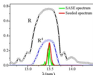
Reflectance of the Mo/Si mirror as function of wavelength for one mirror (R) and four mirrors (R4), compared with first passage SASE oscillator spectrum and seeded spectrum at saturation. Incidence angle: 3 degrees from the normal.
