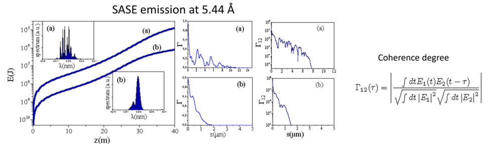
Case (a) refers to the high charge (50pC) multi-spike SASE regime, case (b) to low charge (8pC) single spike regime. Left panel: radiation growth vs undulator coordinate. Right panels: one shot coherence degree and mutual coherence degree between two uncorrelated shots vs  $s=c$  for high (a) and low (b) charge.
