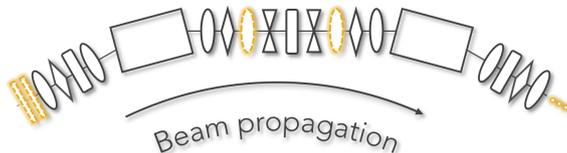
**Figure 2.** Scheme of a right turning DBA. Black parts are present in all the DBAs, the golden parts are the elements present only in the 14<sup>th</sup> DBA that controls the dispersion leak, the final three dots represent the remaining 7 quadrupoles of the the matching line.
